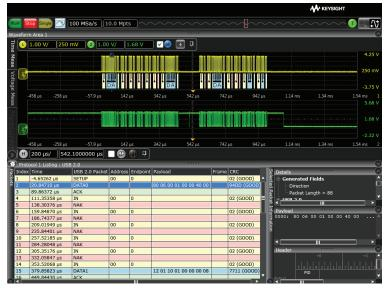
Quickly move between physical and USB high-speed protocol layer information using the time-correlated tracing marker. Display protocol content using embedded decode in the waveform area. Or, see protocol events in a compact listing format using the industry's first scope based multi-tab protocol viewer. For minor tick marks indicate clock transitions. Major tick markets indicate sections of the USB serial packet.
