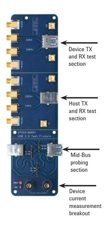
The fixture includes a mid-bus probing section to measure active bus traffic and bus states. It also includes current measurement connections for active power, suspend power and inrush current measurements.
