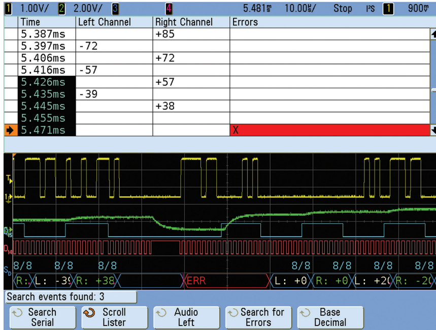
Figure 2. Viewing I 2 S decoded words in the protocol lister display along with automatic search and navigation.
