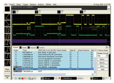
Quickly move between physical and MIPI D-PHY protocol layer information using the time-correlated tracing marker. Display protocol content using embedded decode in the waveform area, Or, see protocol events in a compact listing format. Minor tick marks indicate clock transitions. Major tick marks indicate segments of the serial packet MIPI D-PHY measurements are automatically time-correlated with measurement on other scope channels.
