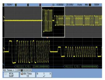
Figure 3. Triggering on a Command Word with a transmit data instruction.
