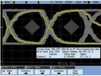
Figure 7. BC to RT OFHEX transformer-coupled input mask test.
