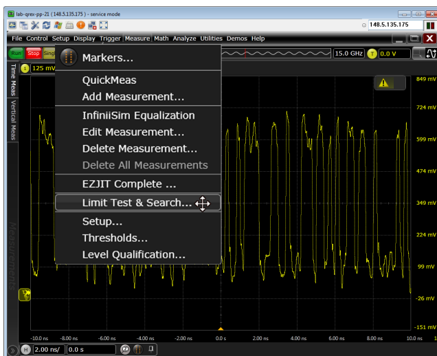
Figure 2. Measurement limit test setup can be found under “limit and test search” in the “acquisition” menu
