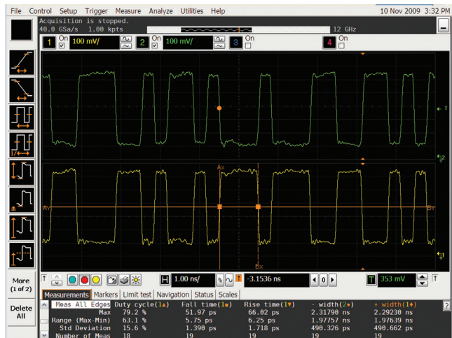
Figure 16. InfiniiScan measurement limit test simultaneously monitoring five different events (positive pulse width, negative pulse width, peak to peak voltage, fall time and rise time) on a single signal.
