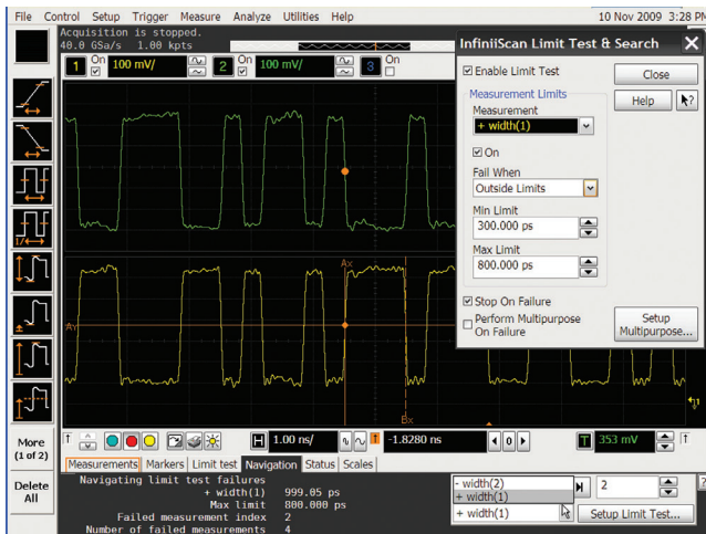
Figure 15. InfiniiScan measurement limit test identifying glitches on two channels simultaneously. Navigation controls (first, previous, next, last) also shown.
