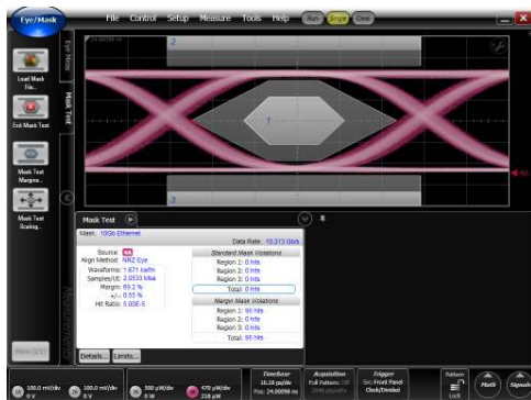
A digital communication analyzer providing fast transmitter characterization using eye diagram analysis, calibrated reference receivers, and automated mask margin measurements
