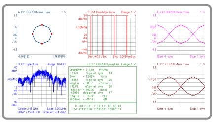
Figure 16. A 2.45-GHz ZigBee transmit PA working in the linear region.
