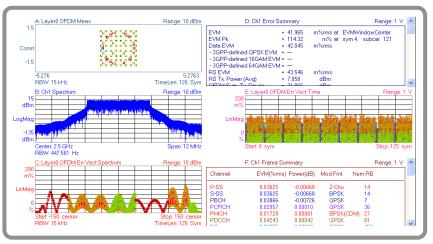
Figure 10. An LTE PA is shown working in its linear region, with a residual EVM < 0.1%, as measured by the independent 89601 VSA measurement software.
