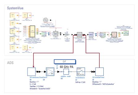
Figure 12. Verifying a 60-GHz PA based on the latest WPAN standard (802.15.3c).
