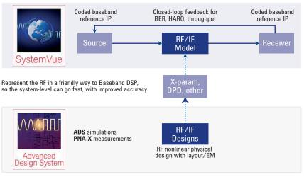
Figure 2. SystemVue and ADS can both export models to each other's environments, allowing faster, offline simulations tailored to that environment.
