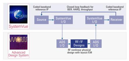
Figure 1. SystemVue can drive ADS in a live co-simulation to achieve higher system-level accuracy and enable more predictive collaboration.
