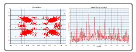
Figure 14. A 60-GHz WPAN PA working in its nonlinear region, with EVM > 20% across a large number of OFDM carriers.
