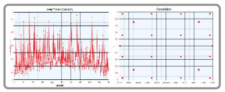
Figure 13. A 60-GHz WPAN PA is shown working in its linear region, with EVM < 0.8% across a large number of individual orthogonal frequency-division multiplexing (OFDM) carriers.
