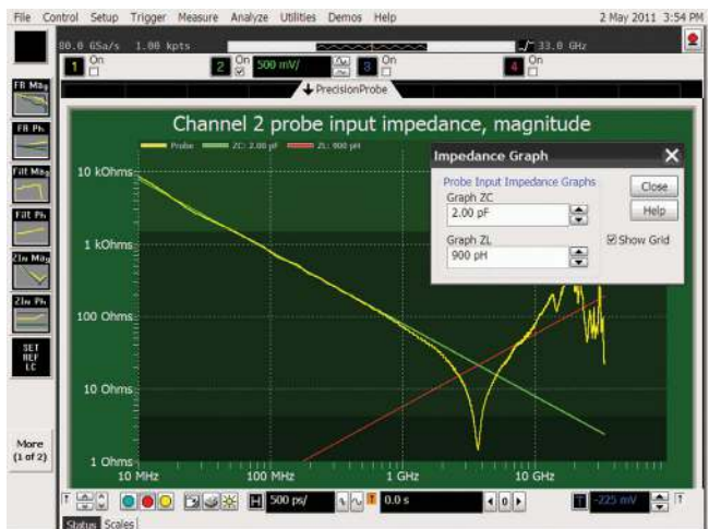
Figure 13: PrecisionProbe properly characterizes a 2 pF capacitor
