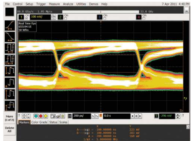
Figure 4: Eye diagram with no correction, notice the minimized eye margins due to fixture loss
