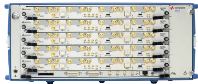
Figure 3. Five Keysight M9703A AXLe 12-bit digitizers installed in the Keysight M9505A 5-slot AXLe chassis to form a 40-channel 12-bit acquisition system.
