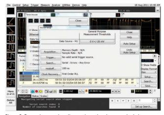
Figure 3. Customize your decoding setting using the manual tab. Image above shows the manual menu option.
