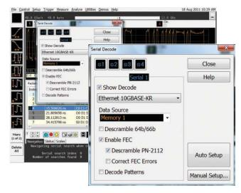
Figure 2. The 64b/66b setup menu includes an "Auto Setup" tab, which enables you to begin decoding 10Gbase-KR signals in less than 30 seconds
