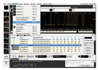
Figure 1. The 64b/66b setup is conveniently located in the "Setup" tab of the Infiniium 90000 and 90000 X-Series oscilloscopes
