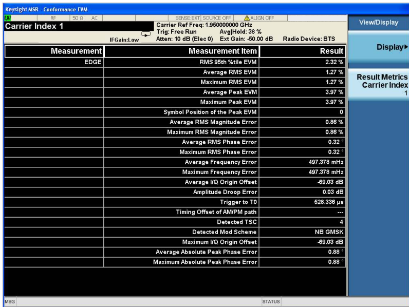
Figure 2. MSR error summary trace showing EVM and frequency error, plus additional error metrics.
