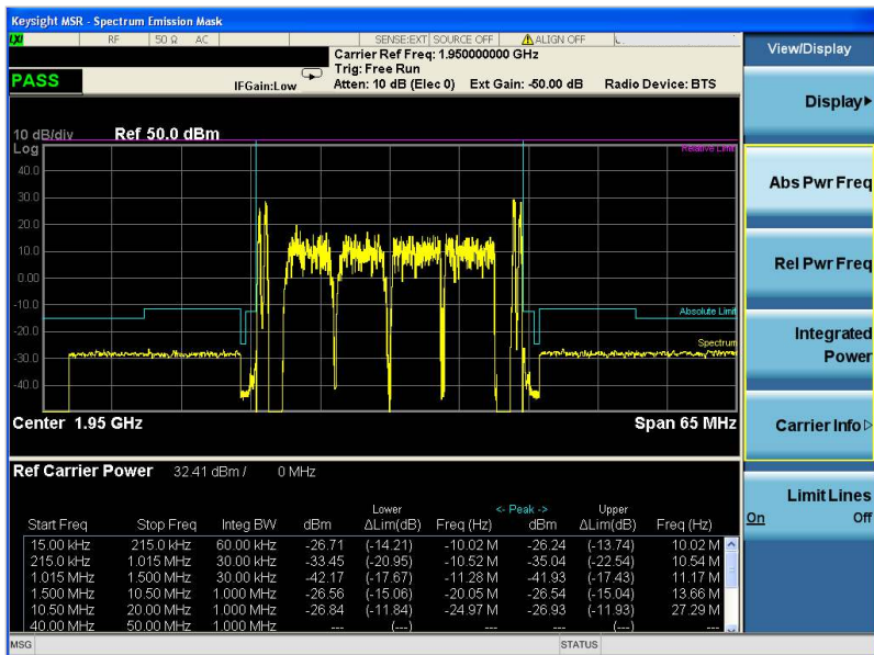
Figure 3. MSR spectrum emissions mask (SEM) measurement for BC2: GSM/EDGE + W-CDMA/HSPA + LTE-FDD with full limit mask according to 3GPP TS 37.141.
