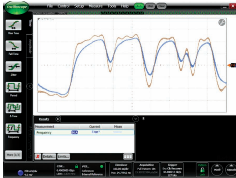
Figure 11. 86100D-SIM InfiniiSim-DCA provides a very fast and easy means to de-embed the effects of the module transmission lines
