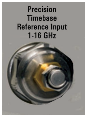
Figure 13. The 86108 Precision timebase reference input
