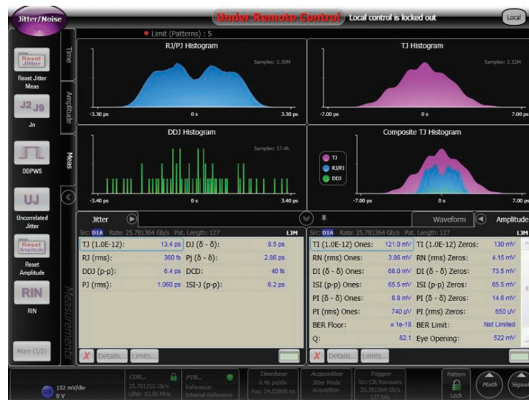
Figure 14. Typical measurement results from use of remote script on data stream at 25.78 Gb/s
