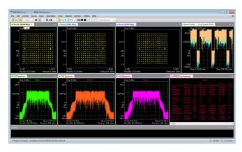
Figure 2. 3-channel 802.11ac analysis using Keysight's 89600 VSA software.
