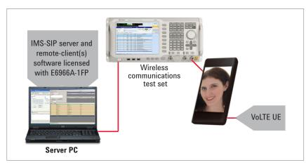
Figure 5. Example test configuration for UE with native client, connecting with an Keysight IMS-SIP server and remote-client software on server PC
