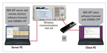
Figure 6. Example test configuration for UE without a native client (requires the addition of a client PC running Keysight IMS-SIP client software)
