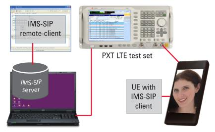
Figure 1. Typical configuration for LTE UE test
