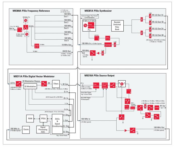
Figure 5. M9381A PXIe vector signal generator block diagram with four modules consisting of the M9301A synthesizer, M9310A source output, M9311A digital vector modulator, and the optional M9300A frequency reference.
