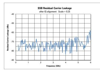
Figure 13. SSB residual carrier leakage.
