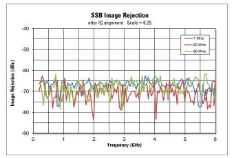
Figure 14. SSB image rejection at 1, 50, and 80 MHz offsets.
