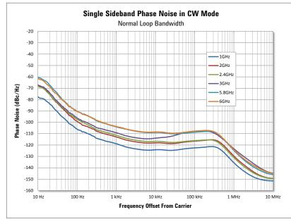
*Figure 11. Single sideband phase noise in normal loop bandwidth, CW mode from 10 Hz to 10 MHz, offset at 1, 2, 2.4, 3, 5.8, and 6 GHz.*
