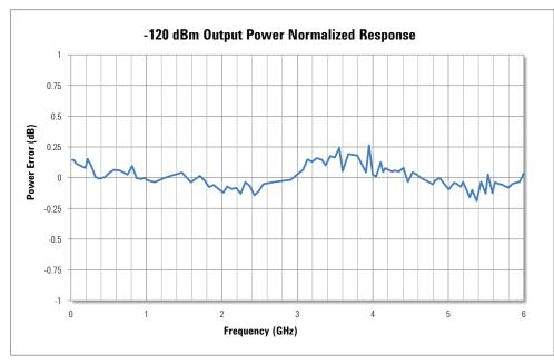
Figure 7. Output power normalized response at -120 dBm.
