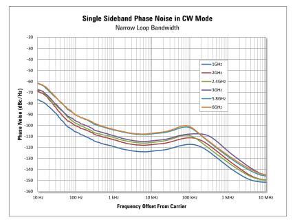
*Figure 12. Single sideband phase noise in narrow loop bandwidth, CW mode from 10 Hz to 10 MHz, offset at 1, 2, 2.4, 3, 5.8, and 6 GHz.*
