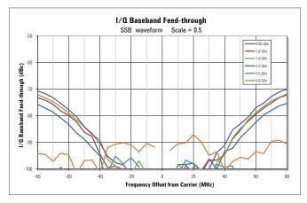
Figure 15. I/Q baseband feed-through at various carrier frequencies.
