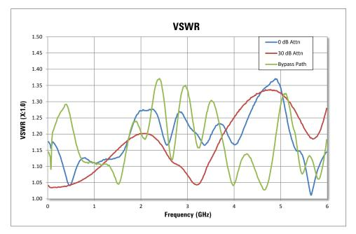
Figure 10. Measured VSWR from 1 MHz to 6 GHz.
