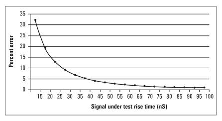
Figure 1. Measured rise time percentage error versus signal under test rise time
