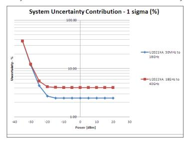
Note: The above graph is valid for conditions of free-run operation, with a signal within the video bandwidth setting on the system. Humidity < 70 %.
