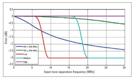
Figure 2. U2021XA/22XA error in peak-to-average measurements for a two-tone input (High, Medium, Low and Off Filters)
