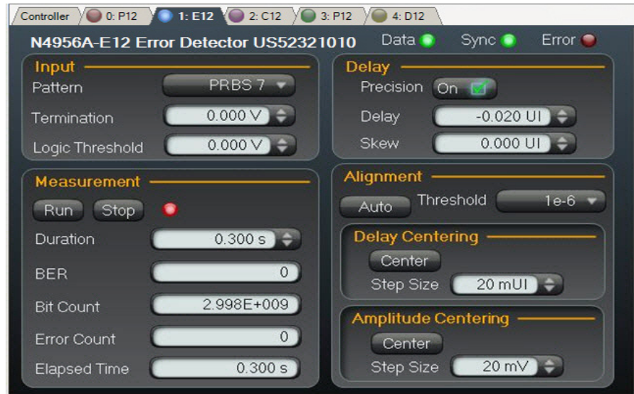
Figure 3. N4965A control panel for easy setup.
