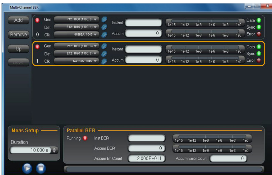
Figure 4. Multi-channel BER measurement results view.
