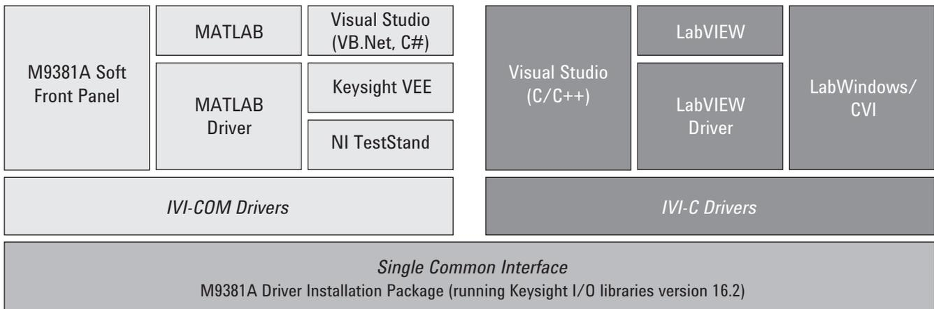
Figure 5. Driver software installed for the M9381A VSG in addition to the instrument library and Keysight I/O Libraries.
