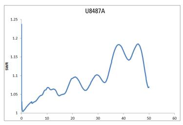
Figure 6. Typical SWR for the AC-coupled U8487A (Option 100)
