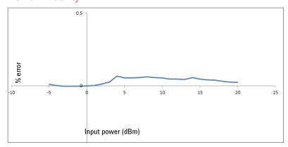
Figure 1. Typical U8480 Series power linearity at 25 °C, after zeroing and calibration with associated measurement uncertainty
