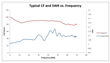
Figure 9. Typical calibration factor (CF) and SWR vs. frequency
