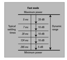
Figure 8. Auto-filter, default resolution, 10 dB decreasing power step
