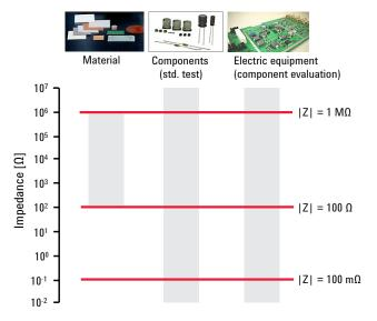
For basic testing or evaluation of electronic components such as capacitors and materials, wide impedance measurement range and test frequency range are required. For example, the high-value capacitance is measured at 120 Hz, and the low-value capacitance is measured at 1 MHz. e.g. 10 mF capacitor:  $|Z| = 133 \text{ m}\Omega \text{ at } 120 \text{ Hz}$ 1 pF capacitor:  $|Z| = 159 \text{ k}\Omega \text{ at } 1 \text{ MHz}$
