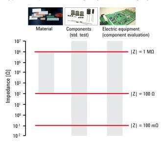
For basic testing or evaluation of electronic components such as capacitors and materials, wide impedance measurement range and test frequency range are required. For example, the high-value capacitance is measured at 120 Hz, and the low-value capacitance is measured at 1 MHz.
