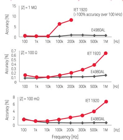
Sources: E4980A/E4980AL Data Sheet 5989-4435EN, 1920 Precision LCR Meter User and Service Manual
