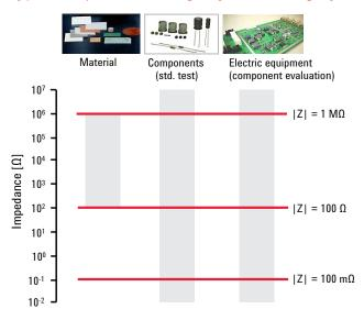
For basic testing or evaluation of electronic components such as capacitors and materials, wide impedance measurement range and test frequency range are required. For example, the high-value capacitance is measured at 120 Hz, and the low-value capacitance is measured at 1 MHz.
