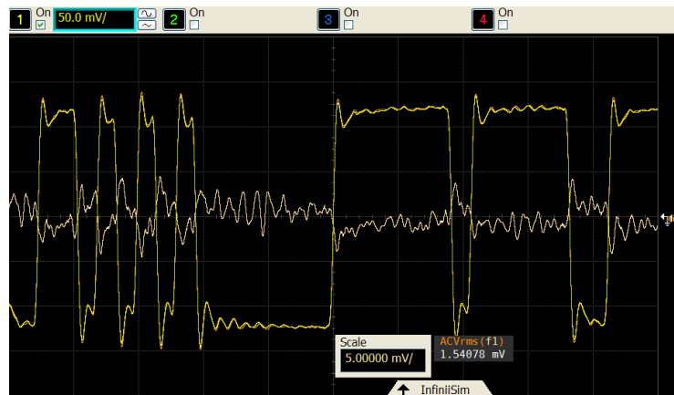
Figure 28. Compensated waveform comparisons. Note that reference and compensated waveforms are overlaid
