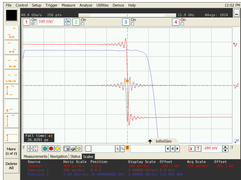
Figure 25. Compensated step response
