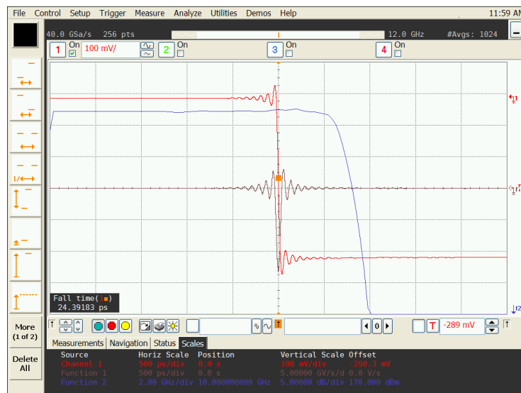
Figure 23. Reference step with derivative and FFT of derivative
