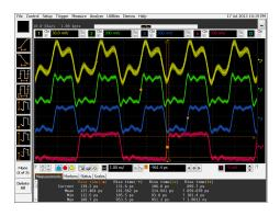
Yellow trace from Tektronix DMAX probing and iCapture output to 4 GHz BW Keysight DSO9404A scope (100 ps input edges). Other traces from coaxial "thru" measurement to scope BNC input. Source: Keysight 8133A pulse generator driving test fixture with common footprint and connection to "thru" signal. Provides a real-time trace capture.
