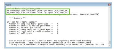
The output message shows that the following nodes "MQ0\_SDR0\_DM" and "MQ0\_SDR0\_ZQ" are not connected to a boundary scan cell or resource.
