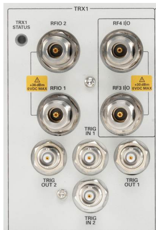
Figure 8. Each TRX in the EXM has its own 4-port RFIO section including two full-duplex ports and two user-configurable half-duplex ports.
