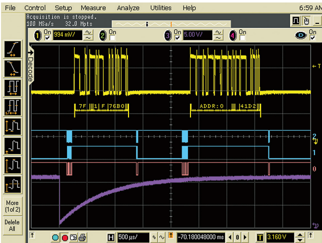
Precise MSO triggering and display Mixed-signal oscilloscope measurement in a mobile system using both digital and analog acquisition channels.
