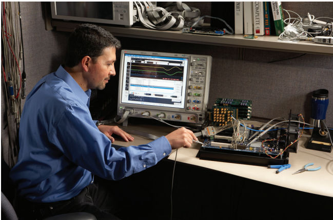
Time correlation with other system activity Protocol measurements are automatically time-correlated with measurements taken on other analog or digital (on MSO models) channels.
