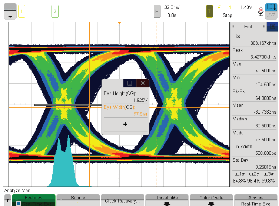
Figure 7: From this display we see a composite view of peak-to-peak edge jitter and noise with extreme positive shifts in the data edges (dark blue traces), which is the cause of the “outliers” revealed in the histogram plot and shows the worst-case eye opening.
