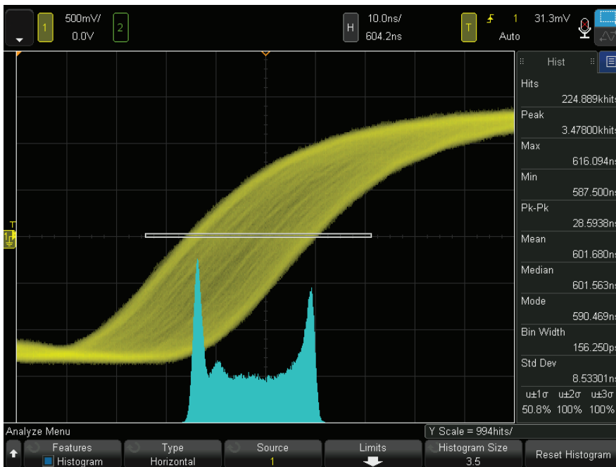
Figure 1: Basic Jitter analysis; viewing repetitive clock jitter with a waveform histogram plot. The histogram (blue) shows that the jitter of the clock (yellow) has bi-modal distribution.
