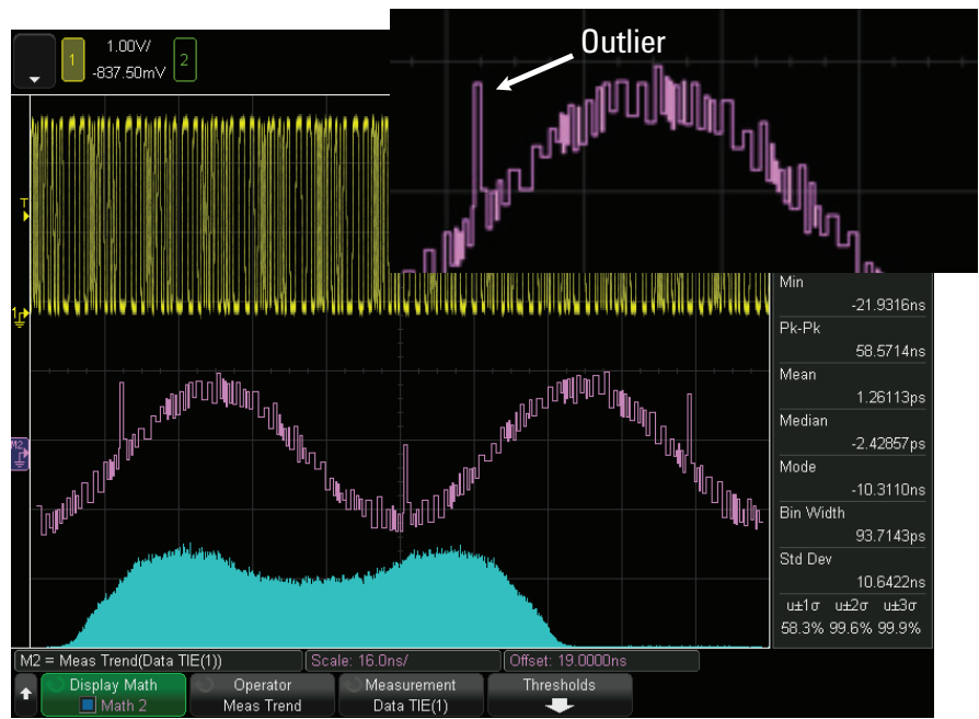
Figure 4: TIE jitter trend waveform shows sinusoidal modulation along with extreme timing errors.
