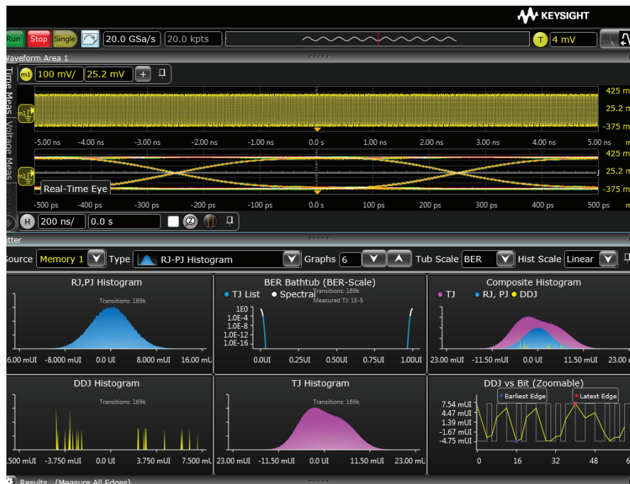
Figure 10: Jitter separation and TJ extrapolation using an Infiniium Series oscilloscope with the EZJIT+ option.
