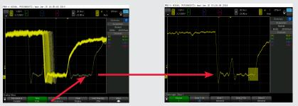
A fast update rate allows you to see an infrequent glitch, but then you want to isolate it. With the 6000 X-Series' hardware zone trigger, you can draw a box to isolate the signal of interest. If you can see it, you can trigger on it.
