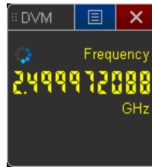
Figure 32. 10-digit counter making precise frequency measurement on a 2.5-GHz signal.
