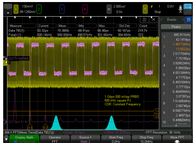
Figure 19. Analyzing periodic jitter (square) on a 1-Gbps PRBS signal.
