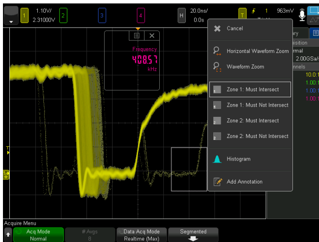
Figure 11. Draw a zone (box) around the anomaly.
