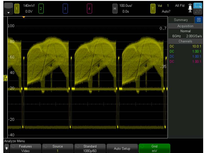
Figure 45. Triggering on a 1080p/60 signal.
