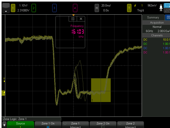
Figure 12. Hardware InfiniiScan Zone triggers immediately.
