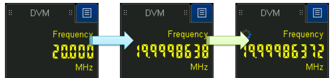
Figure 33. The precise 10-digit counter found the true frequency of a clock to be a little less than 20 MHz.
