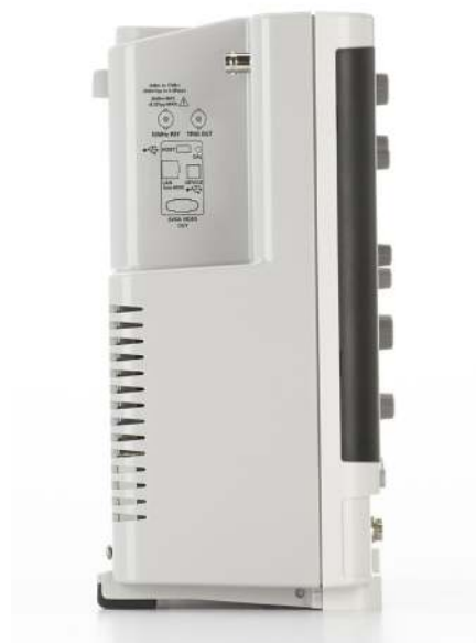
Figure 8. One-gigahertz-per-inch form factor: 6 GHz, 6 inches deep.
