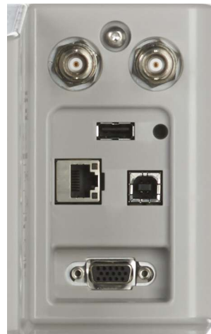
Figure 52. Connectivity section on the back panel.
