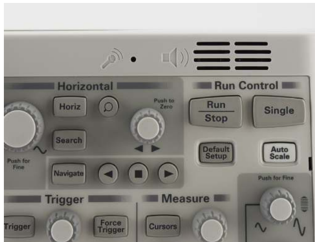
Figure 39. Voice control microphone and speaker.
