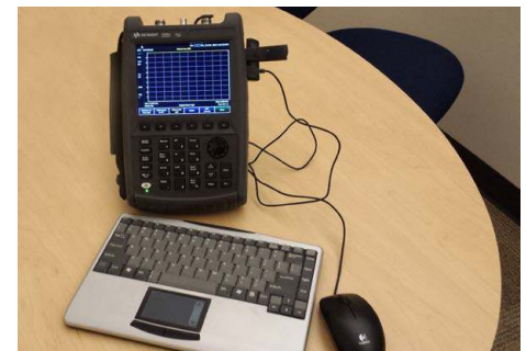
FieldFox with USB keyboard and mouse for easy file naming
