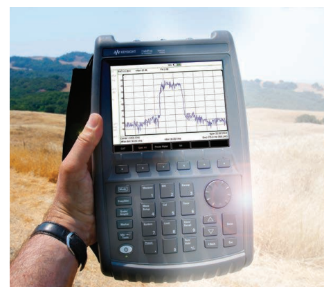
Transflective display makes it easy to read measurements in direct sunlight
