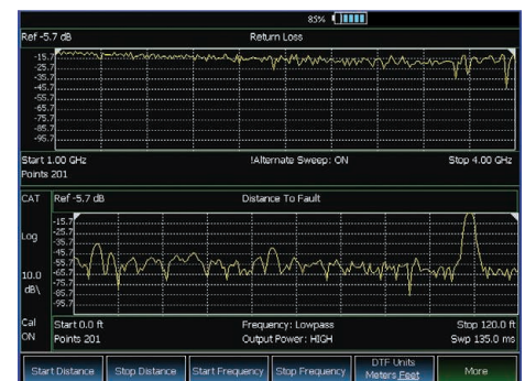
View and control the RL and DTF displays independently
