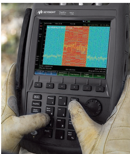
Large buttons make it easy to perform spectrum analysis measurements—even with gloves on
