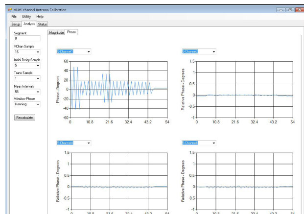
Figure 3. Absolute and relative phase plots, after computing a single I-Q pair for each interval and applying a calibration table
