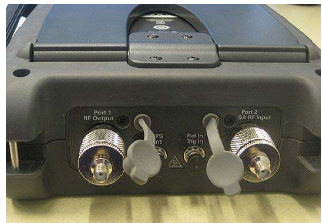
Figure 3. Top view of the FieldFox connection ports with the SMA adapters attached
