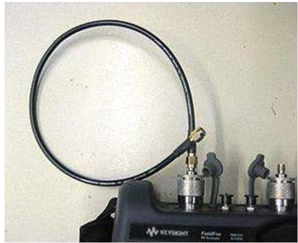
Figure 4. Connection of the RG58C/U coaxial cable to the FieldFox
