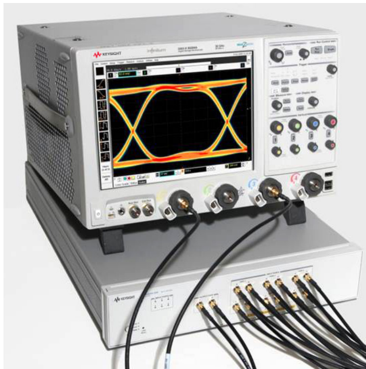
Figure 10. Automated testing for multi-lane digital bus interface through switching solution switch matrix.
