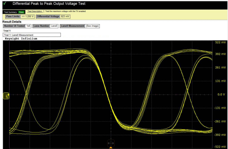
Figure 7. Additional details are available for each test, including the test limits, test description, and test results, including waveforms, if appropriate.
