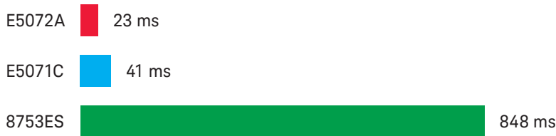
Figure 6. Measurement speed comparison: 1601 points, full 2-port cal, 1 GHz to 1.2 GHz IFBW = 6 kHz (8753ES), 500 kHz (E5071C and E5072A)
