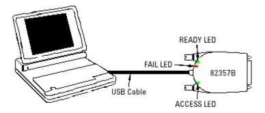
Figure 1-4 Connecting the 82357B to Your PC
