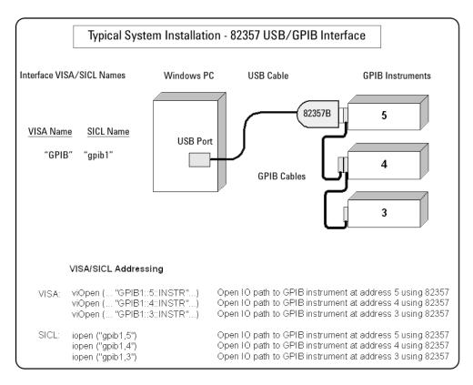
Figure 1-9 Typical System Installation - 82357B USB/GPIB Interface
