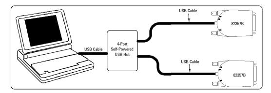
Figure 1-5 Connecting the 82357B to a USB Hub
