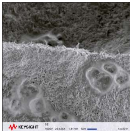
The CNT/chitosan nanocomposite. (Courtesy of University of Hawaii.)
