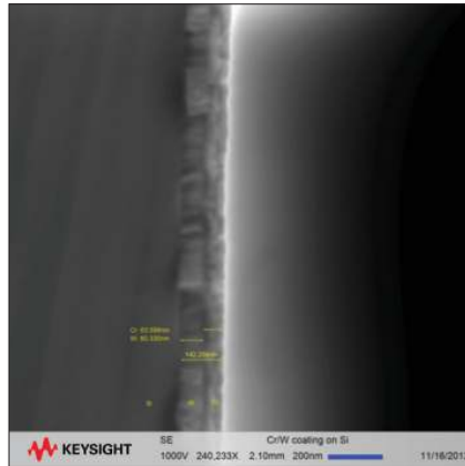
Bilayer thin film coating on Si. (Courtesy of Boise State University).
