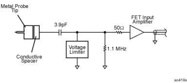
The voltage limiter element has a negligible effect on circuit operation for input voltages within specification. The voltage limiter is a non-linear element: it begins to conduct current at about 2.5 volts. It effectively limits voltages at the amplifier input to less than  $\pm 4$  volts. This prevents amplifier damage from low levels of ESD.
