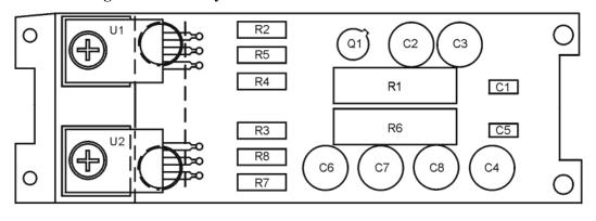
Figure 7-5 A1 Regulator Assembly 85024-63071<sup>1</sup>
