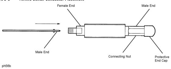
4. Insert the female end of the center conductor into the outer conductor so that the female end of the center conductor is toward the female end of the outer conductor (the end without the connector nut). Refer to Figure 3-8.
