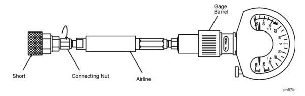
d. Wait approximately 5 minutes for the temperature to stabilize. Do not touch the airline, short, or gage during this time as your body temperature will affect the temperature of the devices.
