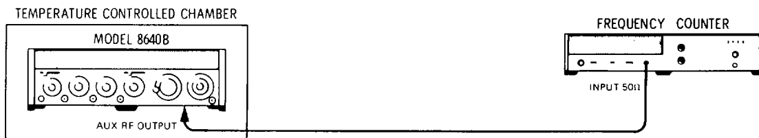
Figure 4-2. Frequency stability vs Temperature Test Setup
