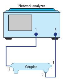
Figure 12. Equipment setup using network analyzer with coupler port 2 and port 3
