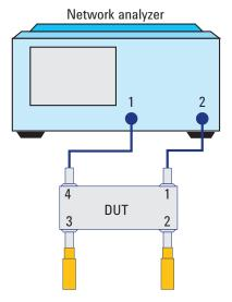
Figure 16. Equipment setup using network analyzer with coupler port 1 and port 4
