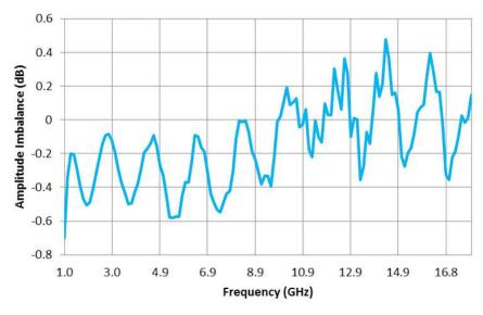
Figure 15. This graph shows the maximum deviation from 0.0 dB reference is approximately –0.7 dB at 1 GHz. The allowable maximum imbalance is 1.0 dB<sup>6</sup>. So the measured amplitude imbalance value –0.7 dB is within the specification.
