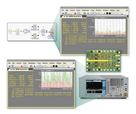
Whether you are analyzing a simulation or physical hardware, the 89600 VSA software tracks expected performance and uncovers errors. Here, the EVM values are only slightly different, but the error vector time trace indicates a filtering problem compared to simulated values.
