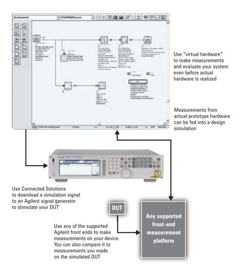
Use the 89600 VSA software and Connected Solutions to create "virtual hardware" where the simulation acts as a missing design block — allowing you to uncover system problems before hardware even exists.
