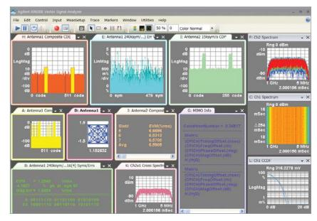
Up to 20 displays each with 20 markers can be viewed per 89600 instance in the simulation design. Innovative display formats, like cumulative history, spectrogram, and digital persistence offer insight into a signal's behavior over time.
