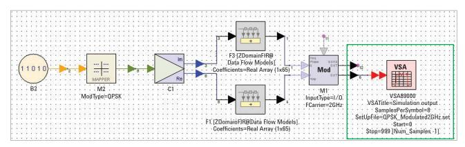
Option 105 provides both a real time source element and visualization sink to add to your simulations. Here the VSA simulation setup includes a few basic parameters and a saved instrument setup file.
