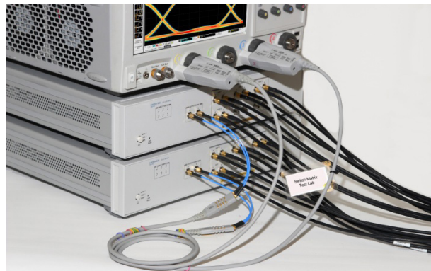
Direct probing test interface
