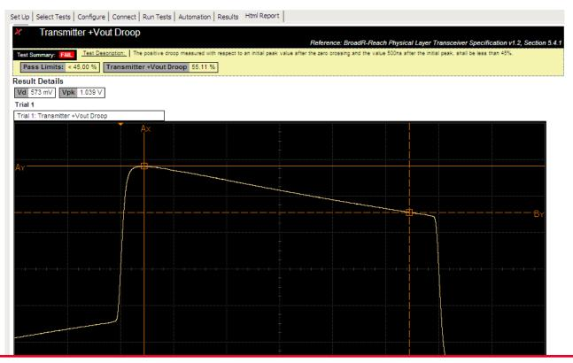
In the report we can display screen shots of the device under test to show how the signal passed or failed. In this case we are showing the Droop test measurement.
