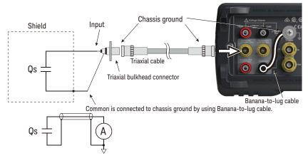
Procedure You can perform the charge measurement as follows. Also see "About Charge Measurement" on page 123.
