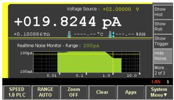
Figure 5-13 shows current noise level when the SPEED (aperture time) of the current measurement is set to 1.0PLC. You can find the following from this graph.
