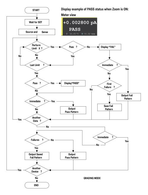
Figure 5-8 Limit Test Flowchart Example for Sorting Mode
