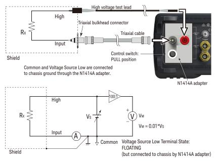
For the floating device measurement, set the N1414A control switch to the PULL position. Also set the voltage source Low terminal state to FLOATING.
