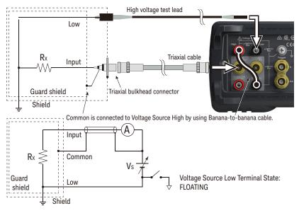
The connection shown in Figure 3-14 applies the voltage to the Common terminal from the Voltage Source. The voltage up to  $\pm 500$  V can be applied to the Common terminal.
