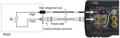
Common is connected to chassis ground by using Banana-to-lug cable.
