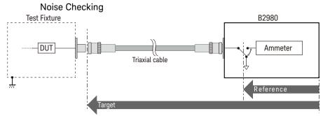
This example confirms if the Triaxial Cable is the noise source.
