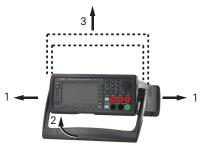
3. Pull outward and then lift the handle upward.
