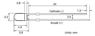
Figure 2-4 Dimensions of the Interlock Switch (Keysight N1254A-402)
