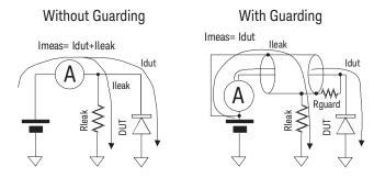
If a dielectric exists between the Input of Ammeter and the other potential, the leakage current flows in accordance with a potential difference and resistance. Guarding technique covers the wire connecting from the Input of Ammeter with a conductor (Guard) that has same potential as Input to cancel the potential difference from the surrounding dielectric so that the leakage current can be
