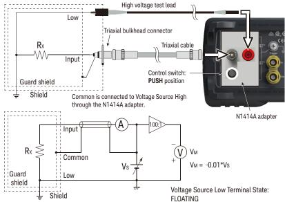
For the grounded device measurement, set the N1414A control switch to the PUSH position. Also set the voltage source Low terminal state to FLOATING.
