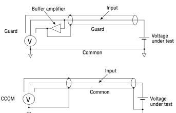
The guarded voltage measurement is effective when the guarded voltmeter indicator turns on. In this setup, the same potential voltage appears at the center conductor (Input) and the inner shield through a buffer amplifier (x1) as shown in Figure 3-9. It is effective for performing voltage measurement accurately.
