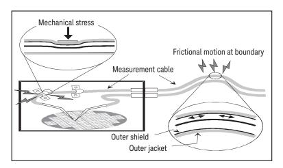
Generally, using the low noise coaxial cable can reduce the noise caused by vibration. Also fixing the cable is effective for preventing it from vibration. Note that applying too much stress to the cable or bending it tightly will have a detrimental effect on the measurements
