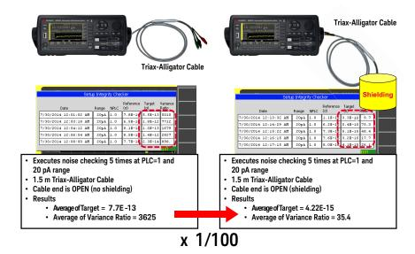
This example compares the case with connecting the Triax-Alligator cable only (the left side in the figure) and the case with connecting the Triax-Alligator cable covered by the shield case that is connected to the chassis (the right side in the figure). In the comparison, the noise checking was performed 5 times and the average of the results is calculated in both cases.
