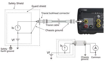
For floating the ammeter, do not connect any cable between Common and chassis ground. See "Common Terminal Connection" on page 92 for more information.
