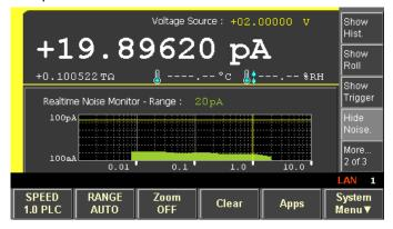
Figure 5-14 shows current noise level when a DUT is connected using shielded wires. You can find that the shielded wires reduce current noise level.
