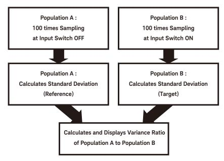
If the one-sided F testing for 95 % reliability is performed on these results and the calculated Variance Ratio is less than 1.4, the population A (Reference), where the input switch is OFF, and the population B (Target), where the input switch is ON, are deemed to be same. That means the noise level of the Target that includes your measurement environment is considered to be the same as that of Reference.
