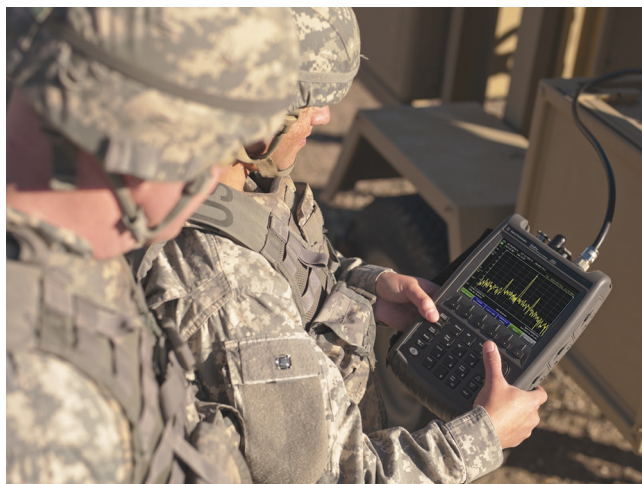
▲ Fig. 1 Agilent’s FieldFox handheld analyzers provide precise microwave measurements in harsh conditions.
