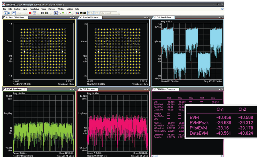
Figure 7. These 89600 traces show the RF MIMO demodulation results at 5.8 GHz: two constellations, two frequency spectra, and the EVM.
