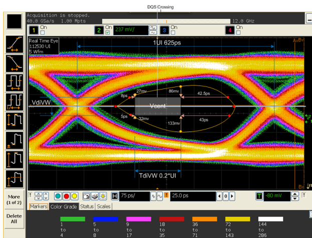
Figure 3. Data Eye with 1E-12 BER
